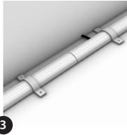
Position additional lengths end to end for seamless, continuous light runs. Only power on once all electrical connections are made and installed by qualified electrician.
