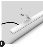
Surface mount with supplied brackets (4 per metre) using corrosion resistant screws that are suitable for surface material and location and ensuring allowance for cable exit.
